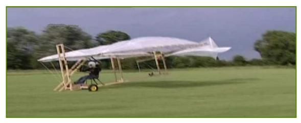
Clearly the authentic Cayley aerofoil was generating lots of lift and the rear end of the machine was nicely airborne, unfortunately causing the nose to dig into the ground, suggesting the machine's centre-of-gravity was too far forward. Some 'empirical redesign' (moving the pilot's seat further back...) and further testing failed to achieve a sufficient improvement; the front end remained stubbornly grounded.
